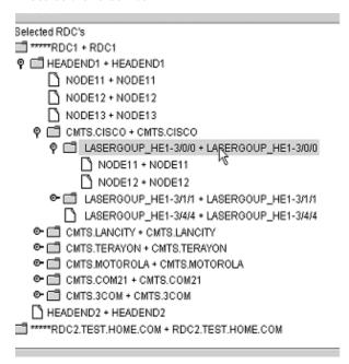
Each level of indentation in the NCP window reflects an item's relationship in the network hierarchy. In the example above, the nodes NODE11, NODE12 and NODE13- along with the CMTS (CMTS.CISCO, etc...)- are indented from HEADEND1. This implies that the indented items are attributes of that headend.
