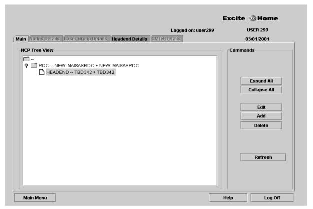
The Main Tab contains the default NCP Tree View window. This window illustrates the hierarchical view of the network topology from the RDC down to the nodes. It displays the relationships between the network's RDCs, headends, nodes, CMTS, and the lasergroups.
